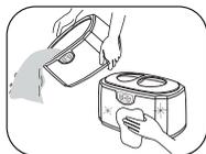
After use, ensure the unit is unplugged. Pour the water away and wipe the stainless steel tank and housing with a clean dry cloth.
