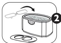
Place the item to be cleaned into the water. Ensure any items with a delicate surface such as glasses/sunglasses lenses are not touching or rubbing the tank walls or base. Ensure the item is immersed as fully as possible, ensuring the water level does not exceed the "MAX" marking.
